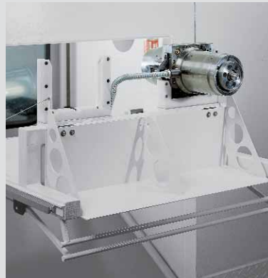
Spindle storage station with finishing spindle.
